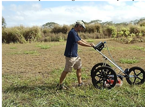
6.30.12 Mike Desilets of Garcia & Associates came with ground-penetrating radar equipment to seek the unseen then shared preliminary findings with Tom...
